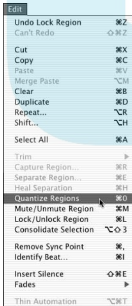
Figure 3-19: The Quantize Region command moves the Start or Synch point of a region to the nearest grid boundary.
